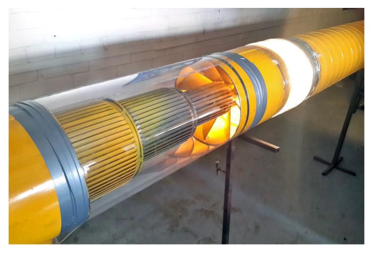
Researchers of the Peter the Great St. Petersburg Polytechnic University (SPbPU) within the framework of Project 5-100 developed a dust collection unit which is capable of the burning metal particles removing from the air flow. According to experts, the equipment allows reducing the fire risks in the industrial enterprises.
