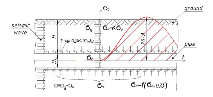
Disregard of the longitudinal stress means that all oil and gas underground pipelines are more susceptible to earthquakes than was initially expected.
